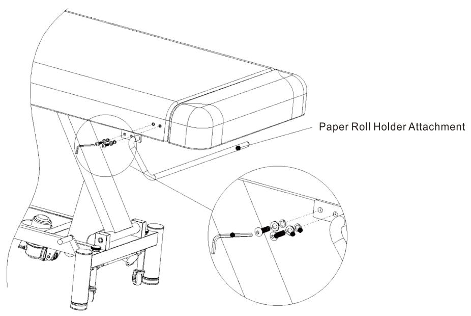
Align Paper Roll Holder onto frame, secure it in place with provided Screws, Washers, Lock Washer and Hex Key.
